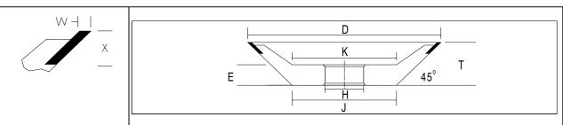
CNC D12V9/45 75-2-10-20 D64-C100 CNC D12V9/45 75-3-10-20 D64-C100 CNC D12V9/45 100-2-10-20 D64-C100 CNC D12V9/45 100-3-10-20 D64-C100 CNC D12V9/45 100-3-10-20 D126-C100 CNC D12V9/45 125-3-10-20 D64-C100 CNC D12V9/45 150-3-10-20 D64-C100 CNC B12V9/45 75-2-10-20 B107-V240 CNC B12V9/45 100-2-10-20 B107-V240 CNC B12V9/45 100-3-15-20 B107-V240 CNC B12V9/45 100-3-15-20 B151-V240 CNC B12V9/45 125-3-15-20 B107-V240 CNC B12V9/45 125-3-15-20 B151-V240 CNC B12V9/45 150-3-10-20 B107-V240
