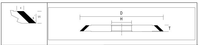
CNC D1V1/10 75-10-5-20 D64-C100 CNC D1V1/10 100-10-5-20 D64-C100 CNC D1V1/10 100-15-5-20 D64-C100 CNC D1V1/20 100-15-5-20 D64-C100 CNC D1V1/30 100-15-5-20 D64-C100 CNC D1V1/45 100-15-5-20 D64-C100 CNC D1V1/45 125-4-6-20 D64-C100 CNC D1V1/20 125-6-5-20 D64-C100 CNC D1V1/10 125-10-5-20 D64-C100 CNC D1V1/20 125-10-5-20 D64-C100 CNC D1V1/20 125-10-5-20 D64-C100 CNC D1V1/20 125-10-5-20 D64-C100
